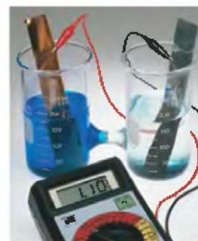
▲ **Figure 20.4** A voltaic cell based on the reaction in Equation 20.7. The left compartment contains 1 M CuSO<sub>4</sub> and a copper electrode. The one on the right contains 1 M ZnSO<sub>4</sub> and a zinc electrode. The solutions are connected by a porous glass disc, which permits contact of the two solutions. The metal electrodes are connected through a voltmeter, which reads the potential of the cell, 1.10 V.
