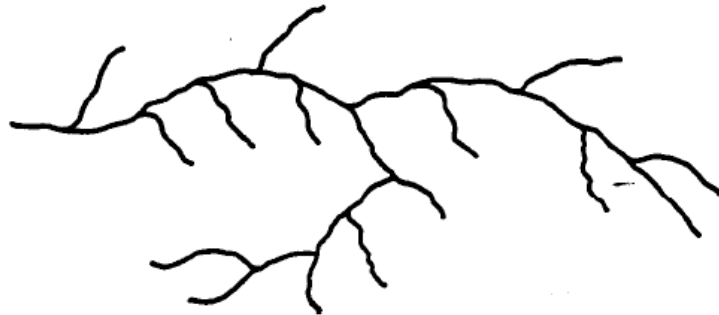
Fig. 4. High-pressure polyethylene, structural principle.
