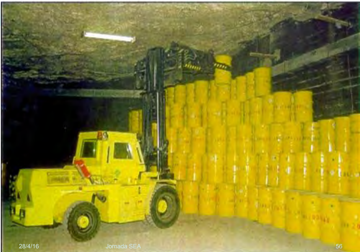
Figure 5-5: Handling of LLW drums in Morsleben Repository
