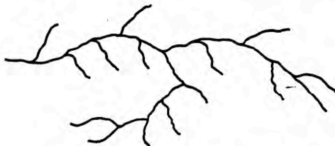
Fig. 4. High-pressure polyethylene, structural principle.
