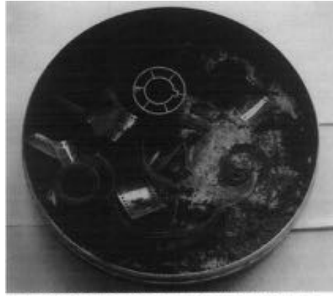
Fig. 1. Naturally aged cellulose nitrate base cinematograph film in a severe state of deterioration, exhibiting brittleness and thickness of emulsion, loss of base and deposition of large volumes of a brown...
