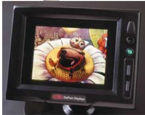
4. Dupont's Olight 4-in. diagonal active-matrix full-color OLED display is
