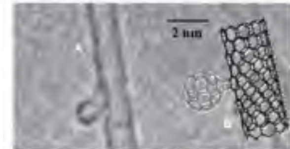
Figure 14 (A) TEM observation of a Nanobud structure, with a fullerene linked to the SWCNT (Reproduced from ref. 58 with permission from the Nature publishing group). (B) Computer generated image of a [50]fullerene linked to the outer surface of the SWCNT by [2-2] cycloaddition.
